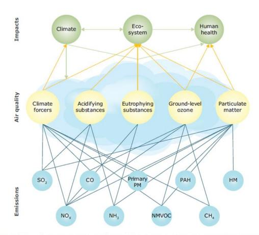
Note: From left to right the pollutants shown are as follows: sulphur dioxide (SO<sub>2</sub>), nitrogen oxides (NO<sub>x</sub>), carbon monoxide (CO), ammonia (NH<sub>3</sub>), particulate matter (PM), non-methane volatile organic compounds (NMVOC), polycyclic aromatic hydrocarbons (PAH), methane (CH<sub>4</sub>), heavy metals (HM).
